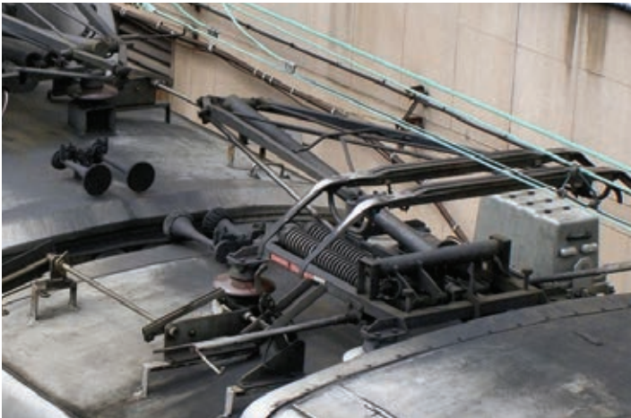
CATHeat installed on METRA Highliner, Chicago IL
