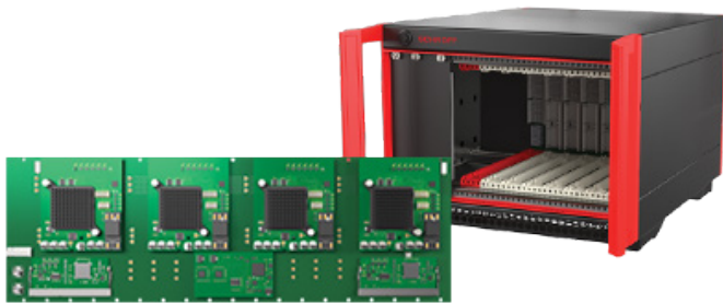
Configuration of a PXI Express backplane
