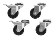
A set of four casters (two locking, two non-locking) that mount directly to the bottom of a frame, 0-mm or 100-mm Solid Base or a Console. (Do not use on plinth bases.) Casters elevate the enclosure 110 mm (4.33) when installed. Caster frames are plated steel with ball-bearing pivots. Caster wheels are made of a black polyamide material. Kit includes M12 mounting hardware. Order separately.
