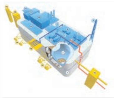
Massive 160m x 39m x 33m LNG Tanks aboard the GBS
