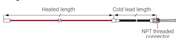
Design D: Dual conductor cable (32, 62 series only)
