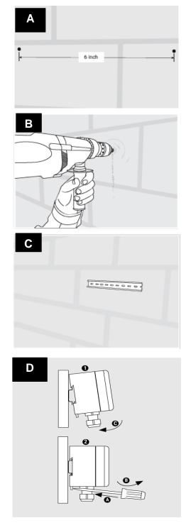
Figure 2.1 – Mounting procedures for the 460 controller
