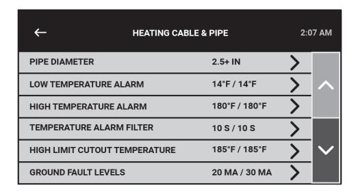
Figure 3.4 - Heating Cable and Pipe Menu
