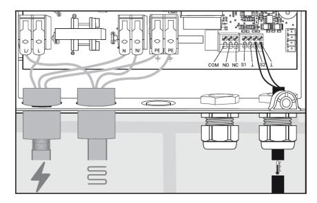
Figure 2.4 - Temperature Sensor Wiring
