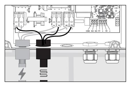
Figure 2.3 - Heating Cable Connection
