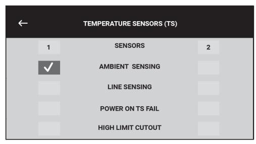
Figure 3.5 - Sensor Setup
