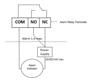
Figure 2.5 - Alarm Wiring
