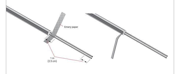
Place a mark at a length "E" (refer to table below) from end of sheath. You will screw the pot on to the sheath so that the back of the pot aligns with the mark.
