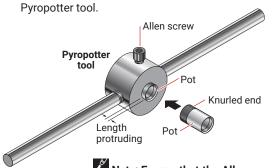
Note: Ensure that the Allen screw is tightened onto the knurled end of the pot.
