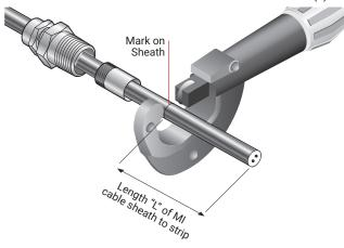
Hold the cable with the handvise behind the score on the sheath. Grip the edge of the sheath between the jaws of the side cutters and twist clockwise (twist counter-clockwise if left-handed), then take a new grip and rotate through a small angle.
