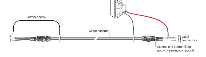
Using a 500-Vdc megohmmeter, check the insulation resistance (IR) of the cable to ensure it is free of grounds and shorts. Check IR between conductor(s) and sheath, and between each pair of conductors. See Appendix A for detailed test procedure and IR test criteria.
