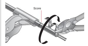
Continue removing the sheath to the score mark. When about to break into the score, bring side cutters to right angle with cable. Finish off with point of side cutters held parallel to the cable. The sheath will peel away leaving a clean cut when the score mark is reached.
