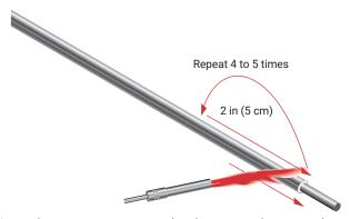
It may be necessary to repeat the above procedure several times to completely remove all moisture from the cable. Allow the cable to cool before repeating.
