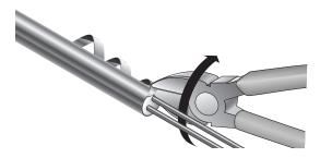
The cable sheath is correctly stripped, with the sheath flared slightly outwards, as shown in (a).
