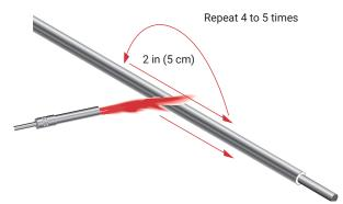
Gradually move the flame toward the end while maintaining the short sweeping motion of the torch. If you heat toward the cable end too quickly you may skip over the moisture and drive it further back into the cable.
