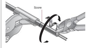
Continue removing the sheath to the score mark. When about to break into the score, bring side cutters to right angle with cable. Finish off with point of side cutters held parallel to the cable. The sheath will peel away leaving a clean cut when the score mark is reached.
