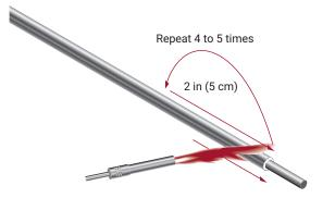
It may be necessary to repeat the above procedure several times to completely remove all moisture from the cable. Allow the cable to cool before repeating. On completion, check IR with a 500-V insulation tester (Megohmmeter).
