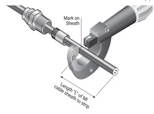
Hold the cable with the handvise behind the score on the sheath. Grip the edge of the sheath between the jaws of the side cutters and twist clockwise (twist counter-clockwise if lefthanded), then take a new grip and rotate through a small angle.
