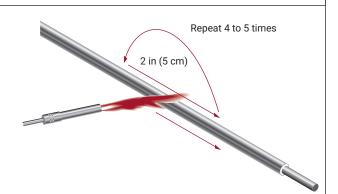
Gradually move the flame toward the end while maintaining the short sweeping motion of the torch. If you heat toward the cable end too quickly you may skip over the moisture and drive it further back into the cable.
