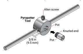
Note: Ensure that the Allen screw is tightened onto the knurled end of the pot
