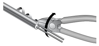
The cable sheath is correctly stripped, with the sheath flared slightly outwards, as shown in (a).
