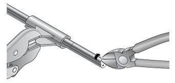
Continue this motion in a series of short "rips", keeping the side cutters at about 45° to the line of the cable, removing sheath spirally. Remove compacted powder insulation to expose conductors.
