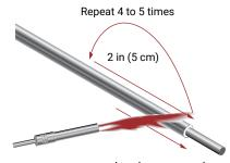
It may be necessary to repeat the above procedure several times to completely remove all moisture from the cable. Allow the cable to cool before repeating.
