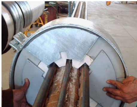
Fig. 14: Pipe Lug on a Traditional Insulated Pipe Anchor (Note the clash between the slots in the lug and the location of the tubes)
