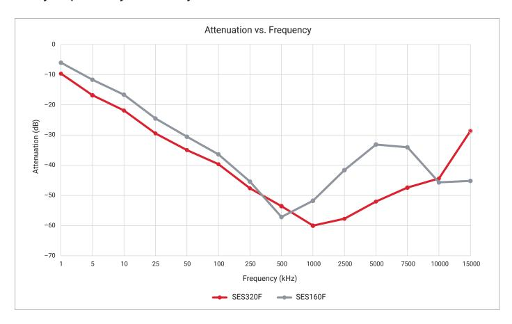
In this test (MIL-STD 220A), the filter is effective at reducing the amplitude of AC voltage signals, especially as a frequency of 500 kHz is approached. Attenuation across a range of frequencies appears to be consistent within the voltage range tested. Frequencies greater than 15 MHz resulted in the sinusoidal signal becoming distorted beyond recognition and the Vpp unable to be measured.
