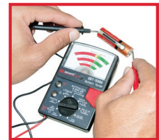
Use test leads to measure battery charge
