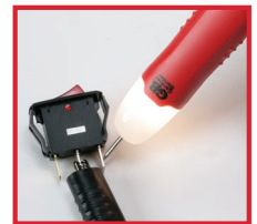
Test continuity of switches
