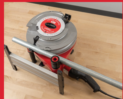
Portable Cyclone can also perform horizontal bends.
