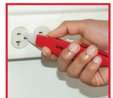
Increasing the sensitivity increases the detection range
