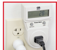
Measure energy consumption for cost planning
