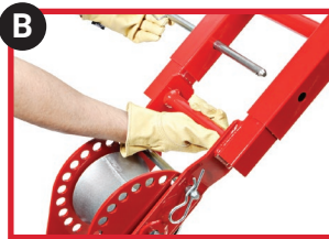
B Extended boom • Allows 12 ft (3.65 m) of cable to be pulled from the conduit to the capstan
