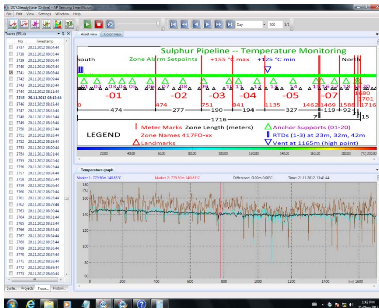
Figure 2. Fiber Optic DTS graphics display.
