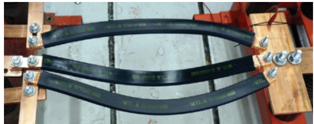
After Short-circuit test
