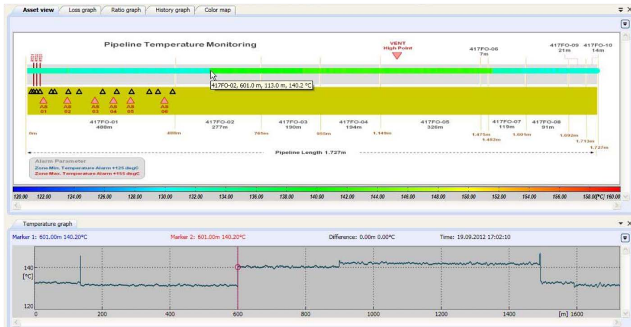
Figure 3. Fiber Optic DTS System Display
