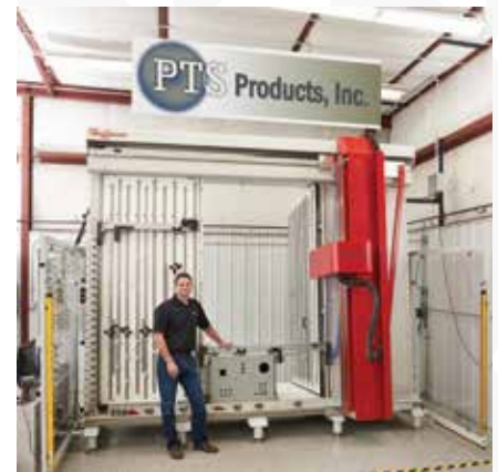
Paul Soberg, founder of Minnesota-based panel shop PTS Products, achieved higher quality and faster turnaround times by automating custom cutouts on its enclosures and back panels using the Steinhauer ModCenter.
